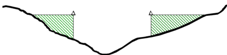
C. Portion of cross sections 2 & 3 that is ineffective for low flow
